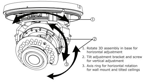
Figure 2-4 Camera adjustment
